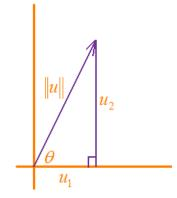
Definition 4: If u is the unit vector such that  $\theta$  is the angle (measured counterclockwise)from the positive x-axis to u, the terminal point of u lies on the unit circle and you have  $u = \langle x, y \rangle = \langle \cos \theta, \sin \theta \rangle = (\cos \theta)i + (\sin \theta)j$
